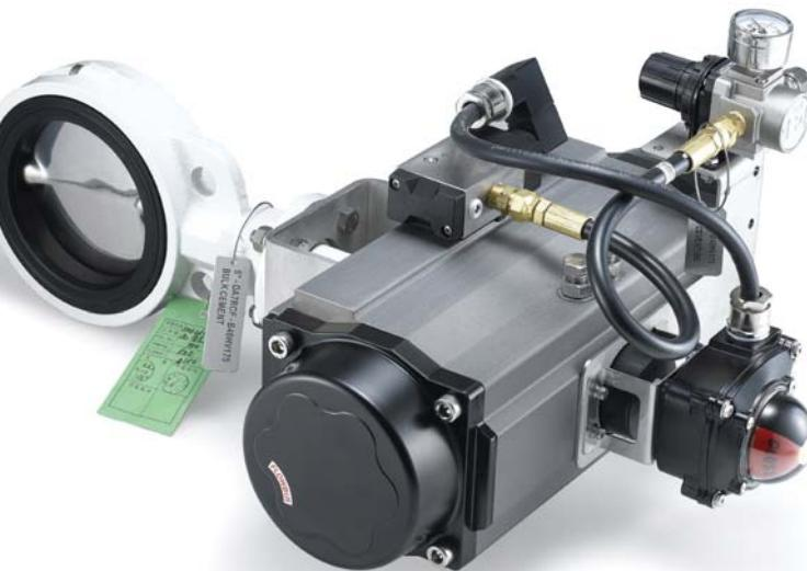
**09** The EPR-Series actuator is available with a declutchable gearbox option. This allows quick and simple operation of the highest torque valves when the air or power supply fails.
